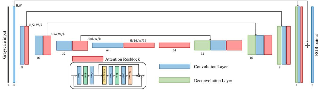
Figure 4. VIDAR’s network architecture.
