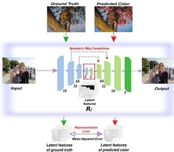
Figure 7. The pksvision\_mm's network structure.
